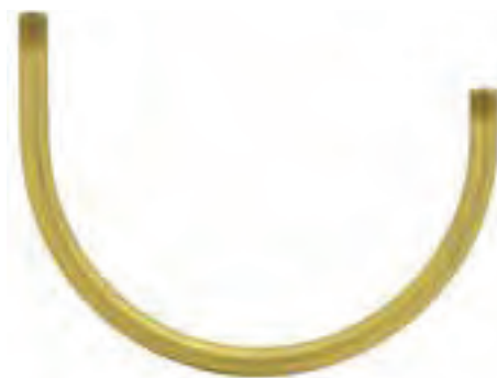
Solid Brass 'U' Arm - Unfinished • Threaded 1/8 IPS • Thread Length 1/4" Each End
