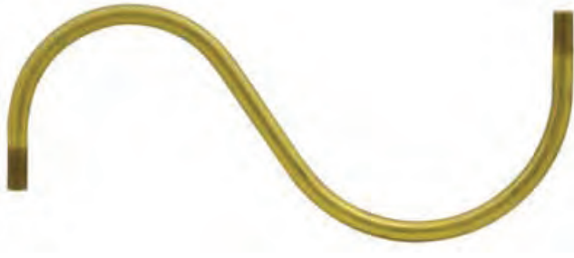
Solid Brass 'S' Arm - Unfinished • Threaded 1/8 IPS • Thread Length 1/2" Each End • 9-1/2" Length X 4-1/4" Height
